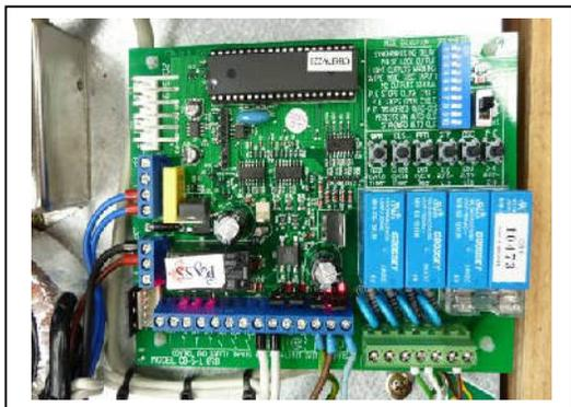
Press the opening button located under the dip switches to begin opening cycle,
