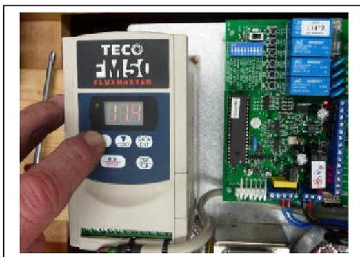
Inverter settings can be adjusted via the keypad i.e. Opening speed, closing speed and ramp times. Automation settings operating modes are able to be adjusted via the CB6 board, refer to manual for further instructions
