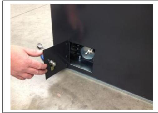
Turn knurled knob anticlockwise approx.  $\frac{1}{2}$  a turn to release. With the clutch door open this disengages the door switch, which in turn inhibits the operation of the operator.
