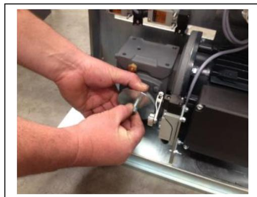
To re-engage the clutch, move the gate by hand into approx. The half way position and turn the knurled knob clockwise until it is very tight.
