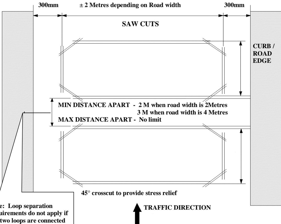
**Note: Loop separation requirements do not apply if the two loops are connected to inputs of a DUAL channel detector. In this case there are no restrictions**
