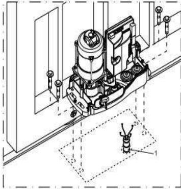
The position of the motor base plate will vary with each installation but in general the base plate needs to be 40mm TO 50mm from the side face of your gate. The height will be determined by your site conditions and gate structure.
