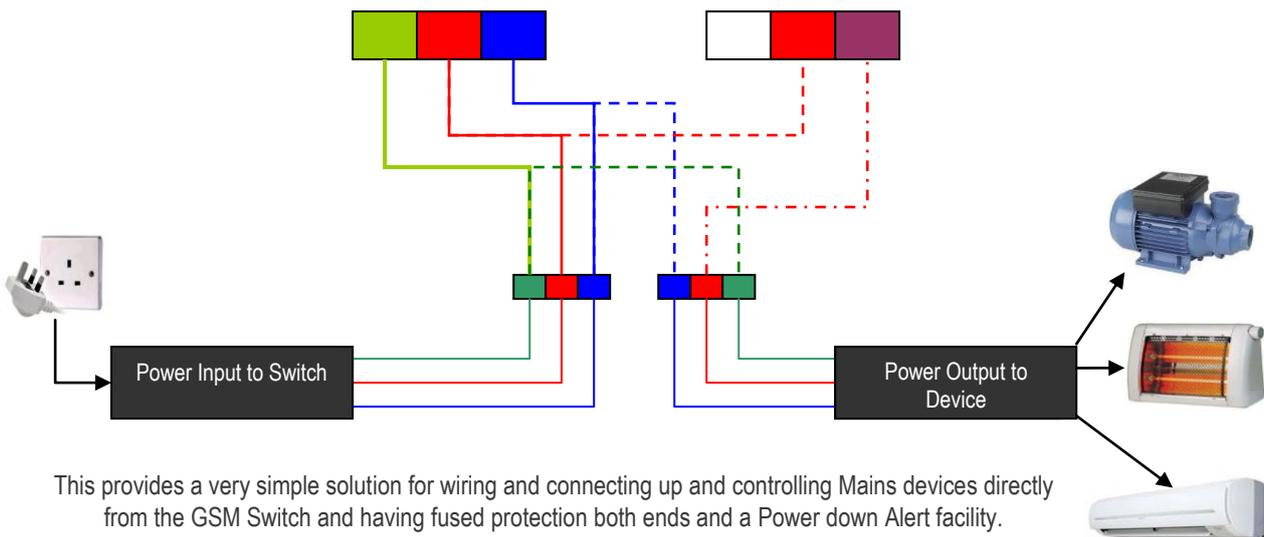
This provides a very simple solution for wiring and connecting up and controlling Mains devices directly from the GSM Switch and having fused protection both ends and a Power down Alert facility.
